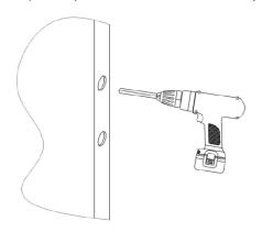
3b. Drill out the main WPT pocket to a minimum depth of 1-7/8" (48mm), and diameter of 1" (25mm)
