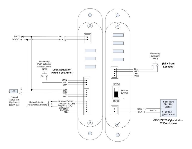
7. Mount both WPT units using the appropriate screws. Apply continuous power to the frame side. If using a momentary switch to activate the lock, hold for a second or two, then release. Power will be provided to the lock for approximately 4 seconds.
