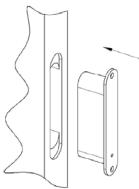
3e. For the door side unit, drill a wiring channel to the electrified device to be powered.
