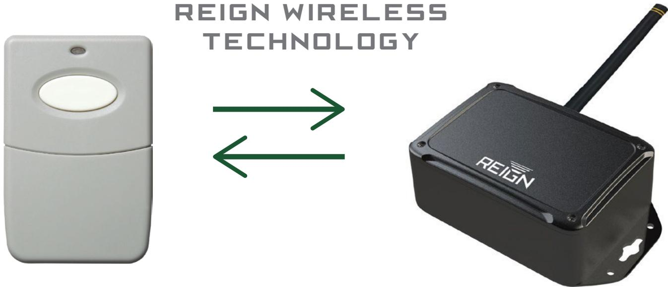
The Reign TX-100-NC & XRE-100 transmitter/receiver kit is a revolutionary product. This product allows for wirelessly triggering a relay through a battery powered hand held transmitter with extreme range, no line-of-sight wireless technology.
