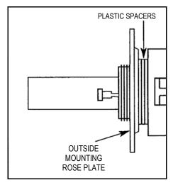
FIG. 9: ADJUST DOOR THICKNESS
