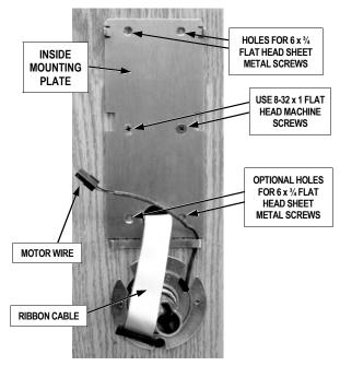
FIG. 13: INSIDE MOUNTING PLATE INSTALLATION
