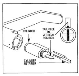
FIG. 20: STANDARD CYLINDER-LEVER, TAILPIECE AND RETAINER.
