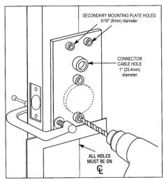
FIG. 2: ALARM LOCK INSTALLATION JIG
