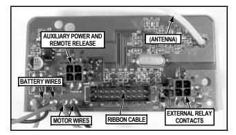
FIG. 14: RECEPTACLES LOCATED IN THE INSIDE HOUSING
