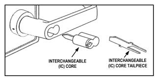
FIG. 22: INSTALL INTERCHANGEABLE (IC) CORE
