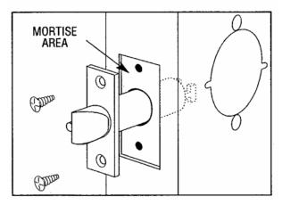
FIG. 3: LATCH INSTALLATION
