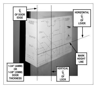
FIG. 1: FOLD AND PLACE TEMPLATE ON DOOR
