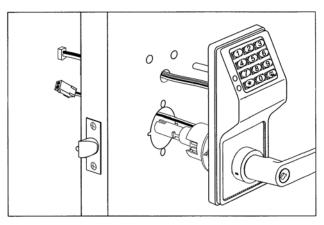
FIG. 7: INSTALL OUTSIDE LOCK BODY (Lever, Housing & Lock body)
