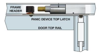
Top Latch Release for Dor-O-Matic and Kawneer Vertical Rod Exit Devices. The **PBD2090A PanicLok** permits access control and remote timer control of narrow stile glass doors equipped with Dor-O-Matic or Kawneer concealed vertical rod exit devices.
