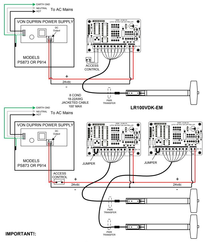
Power the LR100 modules using the MAIN OUTPUT terminals. The zone controller cards are not required and can damage the latch retraction units if used.
