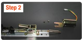
Remove the solenoid from the base rail by removing two Philip screws.
