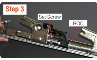
Then turn the device on its side and unfasten the set screw in order to remove the rod. To remove the rod unscrew. (Suggest to use Pliers to remove). \* Note: When removing the rod it may break off.
