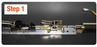
The device should be completely removed from the door, the rail and push pad in order to worked correctly and placed on a work bench or flat surface. As shown.
