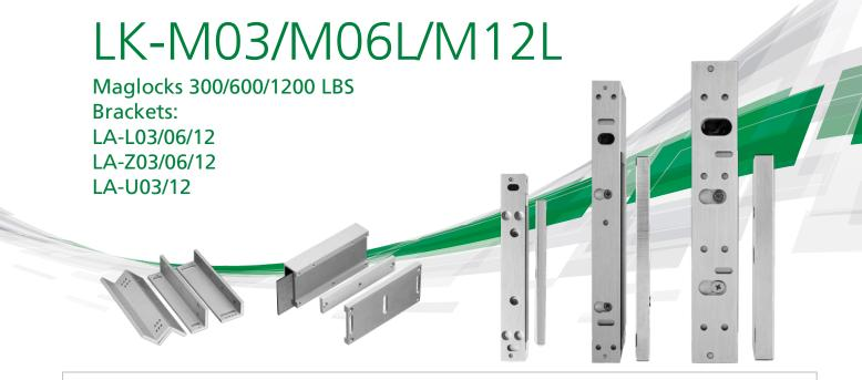
Rosslare's LK-M03/M06L/M12L high quality magnetic locks are ideal for secure applications where access is restricted, such as office buildings, hospitals, and airports. They have a holding force of 300/600/1200 pounds, respectively, and are easy to install. The attractively designed Maglocks are surface mounted, operate on dual voltage, 12 VDC or 24 VDC, and have low current consumption. These Maglocks are compatible with EN and UL standards.
