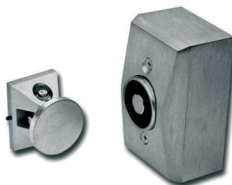
The LCN SEM7800 Series are heavy duty, electrically controlled door holding magnets. Magnets are fail safe and hold until the current is interrupted. A manual door closer is used to control and close the door. A choice of floor, recessed wall, or surface mounted wall magnets are available.
