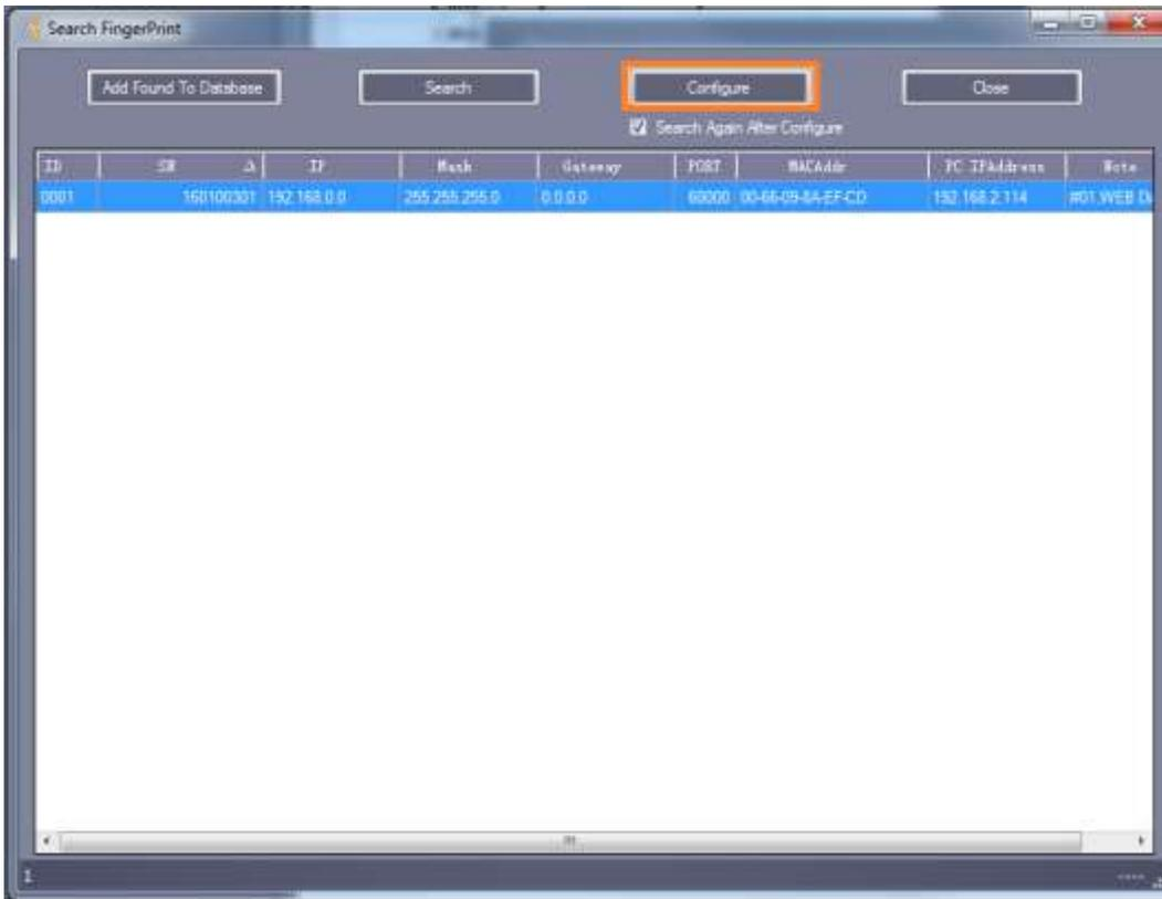
10. Input an appropriate "IP address" and "Subnet Mask" for the reader then click "OK"
