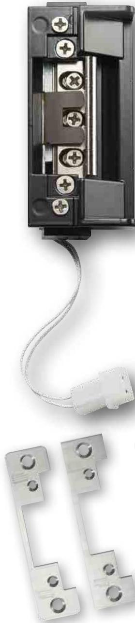
Designed for medium-duty applications, the all-in-one AES-200 offers dual voltage and field selectable fail secure/fail safe operation. Deep latch cavity accommodates cylindrical locksets with a 5/8" throw in steel, wood or aluminum frames. Easy to install and connect.
