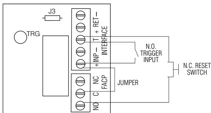
**Fig. 6** Normally Closed - Non-Latching FACP trigger input:
