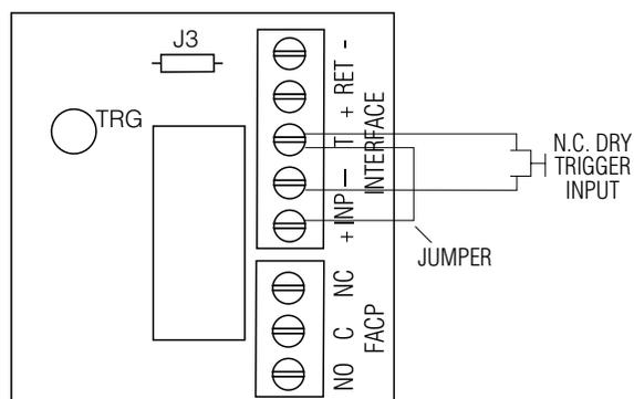
**Fig. 7** Normally Closed - Latching FACP trigger input with reset:
