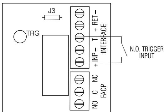
**Fig. 5** Normally Open FACP Latching trigger input with reset:
