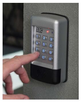
The SDC EntryCheck™ series consists of stand alone digital keypads designed to control access of a single entry point for facilities with up to 500 users. Each user is assigned a personal identification number (PIN). Keypad entry of a valid one to six digit code activates one or both of the output relays which releases an electric door lock. Optional Prox Readers are available for selective models. Many models are now available with industry standard Wiegand 26 bit data transfer.
