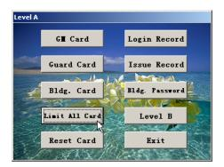
Insert a new card into the encoder and click 'Limit All Card' to issue. The Limit All Card can make all of the former Guest Cards invalid. When you insert it into a lock, the Guest Cards issued and ever used on this lock will be invalid and cannot open this lock.
