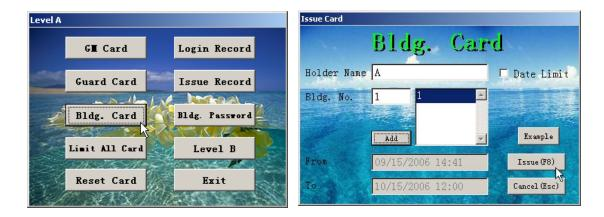
Insert a new card into the encoder, click 'Bldg. Card', input holder name and Bldg. No., then click 'Issue' to make a Bldg. Card. (The Bldg. Card can open all the locks of the hotel except those locks with deadbolt in work.)
