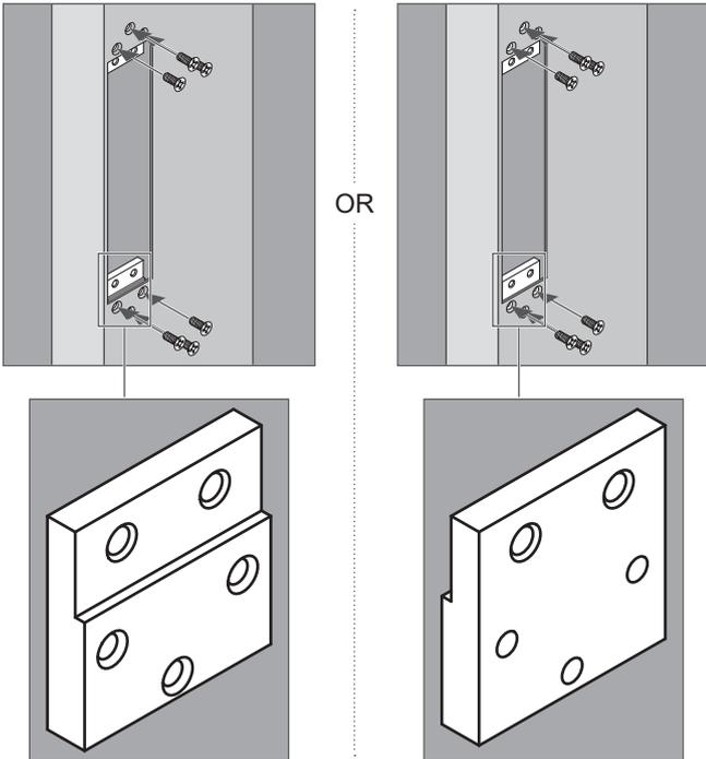
1b Install magnet into frame.
