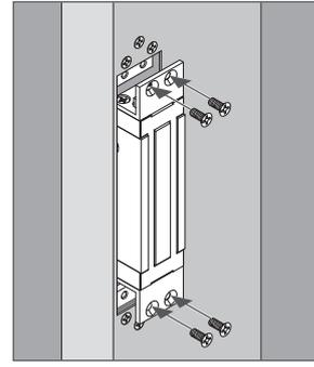
1c Magnet should be completely flush with frame.
