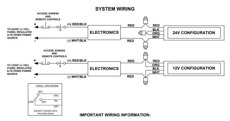
Use the system wiring diagram to configure the EMLock for 12 VDC or 24 VDC operation.
